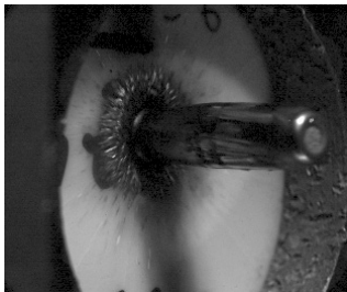
Ballistic test* of Al_2O_3 ceramics in front of aluminum backing.
